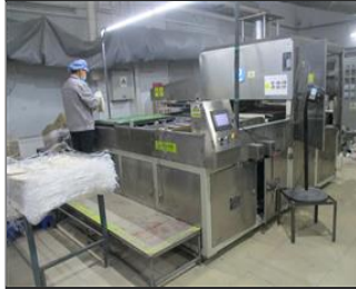
Photo of the inside of the main production hall 9. Edge cutting section.JPG
